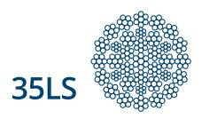
35LS is a conventional low rotation resistant rope consisting of three layers of strands the inner two layers spun in the opposite direction to the outer layer of strands manufactured in accordance with EN 12385.
