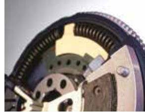
Clutch springs: high shear yield strength and low weight
