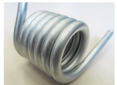
Wrapping test: 6mm Bezinox ® wire wrapped on a 18mm mandrel
